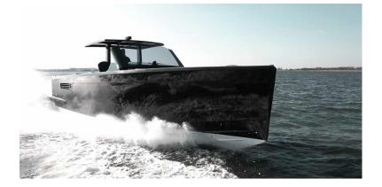
IPS drives and a Joystick make this Yacht very easy to maneuver. One person alone can handle the boat comfortably. The fuel efficient Volvo Penta IPS engines give you a cruising range of over 200 nautical miles at 25 Knots. The choices are IPS 500 or IPS 600, the main difference being the top speed. The IPS 600 will clock 40Knots. The Fjord 42' Open feels solid and stable at any speed resulting in a comfortable and relaxing ride.
